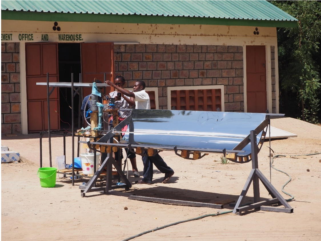
Figure 1: Locally built solar thermal desalinator, Lodwar, Kenya (December 2018)
